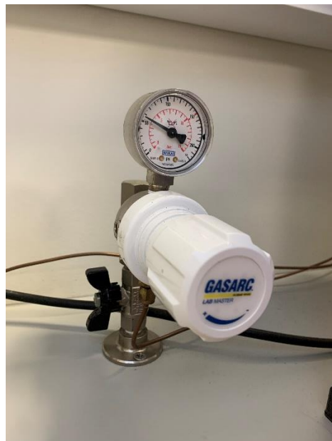
Figure 2: Butterfly valve on the gas regulator in the closed position
