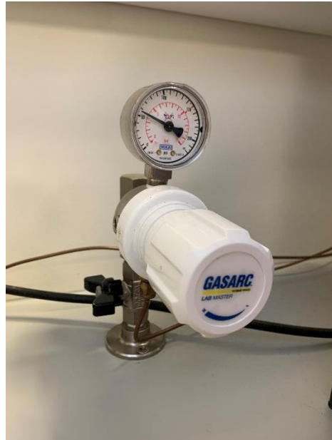
Figure 1: Butterfly valve on the gas regulator in the closed position
